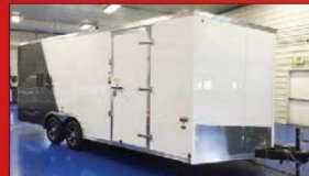
2011 Mettler Slope Nose 20ft Car Hauler - Heavy Duty Ramp Dr. 80" At Rear Dr. Full Luan Backed Roof on 16" Ctrs, 7" 2" Int. Height, 16" On Center Walls, Roof Vent. 6" I-Beam Frame, 2-Tech Chassis Protection, 7,000 lb GVW. Great For Side By Sides. See Mettler's ad inside. 814-789-3726 www.mettlerauto.com
